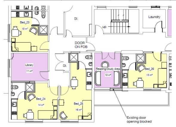
Extract from part of the Proposed First Floor Plan (to show typical apartment layout)
